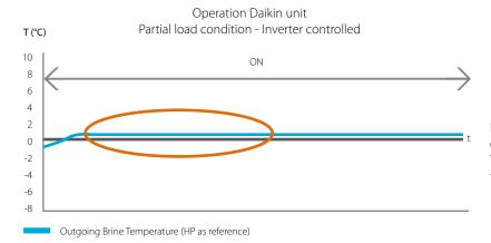
Daikin's inverter technology produces a stable outgoing brine temperature of around 0°C. This higher and more constant evaporating temperature leads to greater operating efficiencies.
